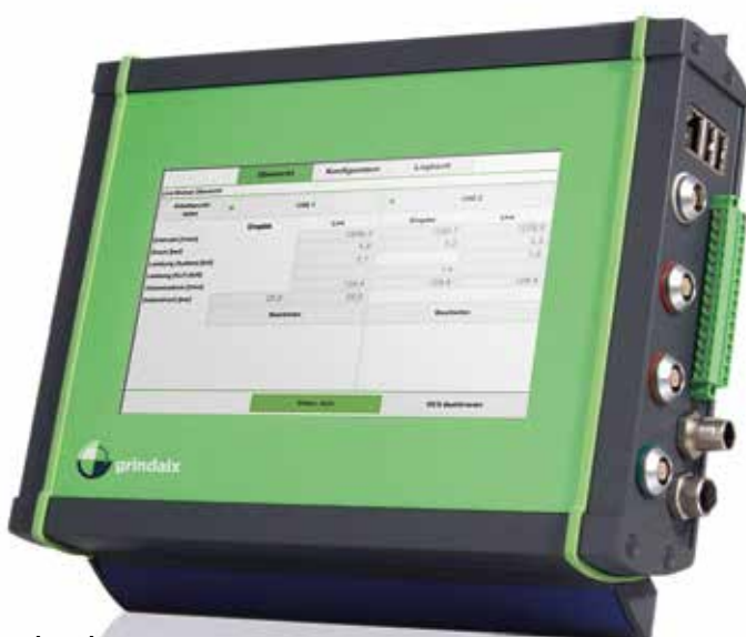
Alustyle Resistive touch screen under a continuous membrane.
