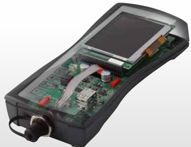
BOS-Streamline Display combined with customised membrane keypad.
