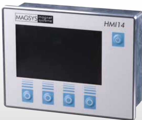
BoTouch Aluminium Profile keypad (illuminated) with resistive touch screen.
